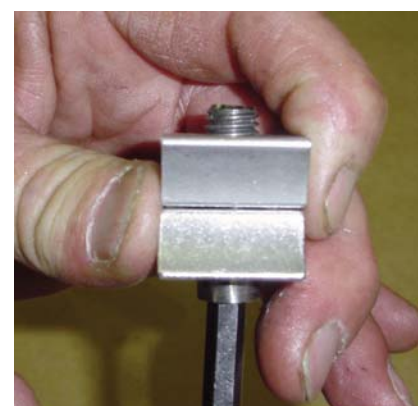
Sandwich spring between recessed portions of pawls. Completely tighten set screw. Keep pawls even.
