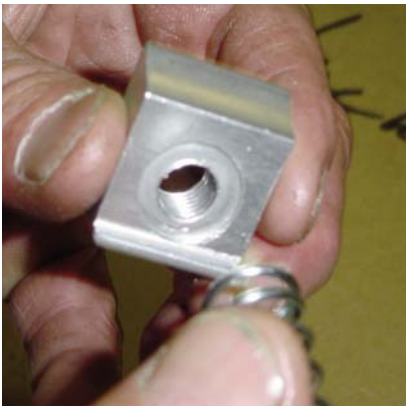
Sandwich spring between recessed portions of pawls. Completely tighten set screw. Keep pawls even.
