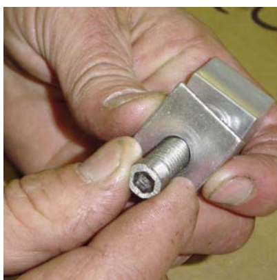
Sandwich spring between recessed portions of pawls. Completely tighten set screw. Keep pawls even.
