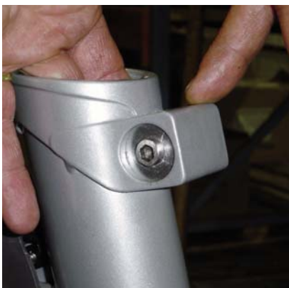
Insert new pawls, keep bolt head on large hole side. Make sure pawl is pushed back and completely remove set screw.
