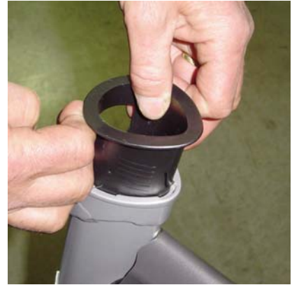
Remove plastic sleeve(push pawls towards front if needed)
