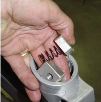
Used supplied allen wrench to carefully remove pawls, spring and shim(on back wall). Avoid dropping parts into bottom of tube.
