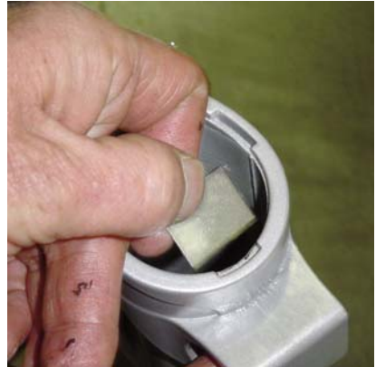
Used supplied allen wrench to carefully remove pawls, spring and shim(on back wall). Avoid dropping parts into bottom of tube.
