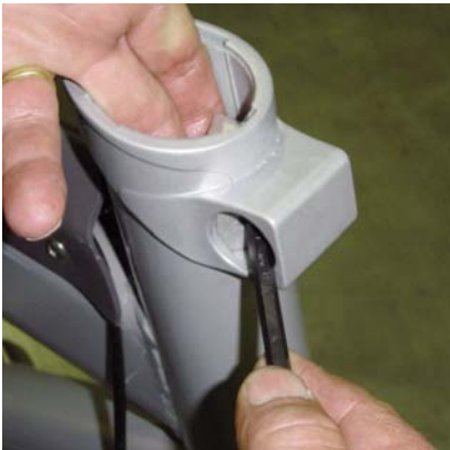
Used supplied allen wrench to carefully remove pawls, spring and shim(on back wall). Avoid dropping parts into bottom of tube.
