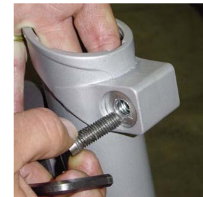
Insert new pawls, keep bolt head on large hole side. Make sure pawl is pushed back and completely remove set screw.
