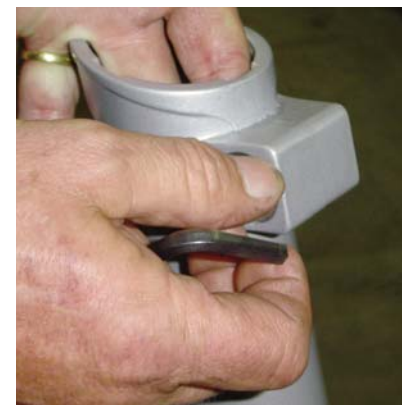
Insert new pawls, keep bolt head on large hole side. Make sure pawl is pushed back and completely remove set screw.
